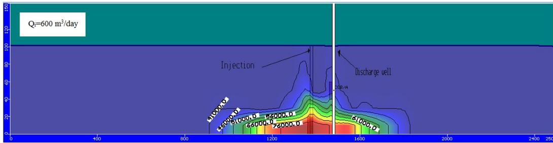
**Fig. 7. Salt concentration distributions along x-z vertical plane after 10 years of simulation for injection rates 600 m<sup>3</sup>/day at S=100 m**
