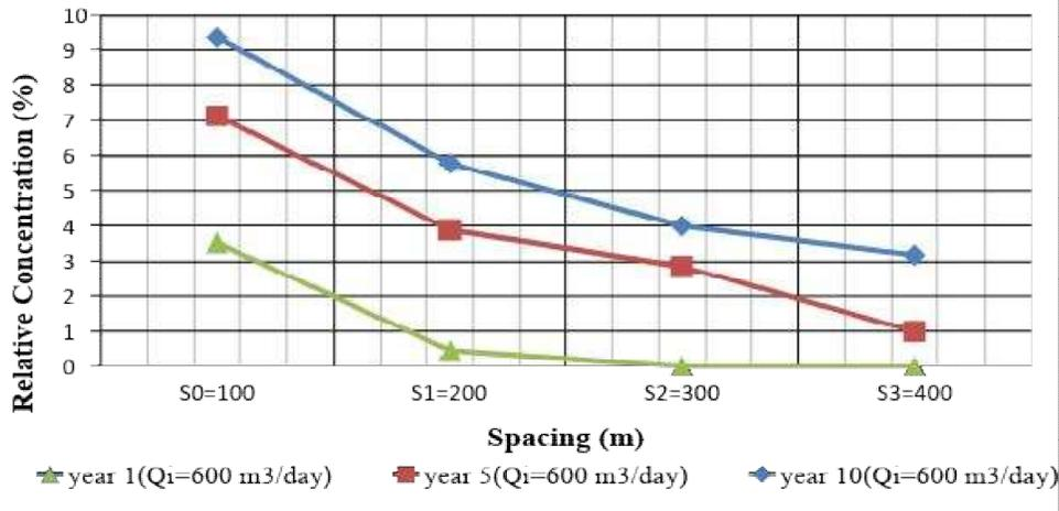
Fig. 6. Design chart for Q<sub>i</sub>=600 m<sup>3</sup>/day after 1, 5, 10 years of simulation
